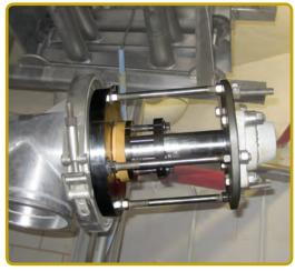
MECO SEAL ON INCLINED PACKAGING SCREW
