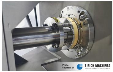
Figure 2. The OFS Type-2 seal model installed on a dry powder blender. Source: MECO Seal
