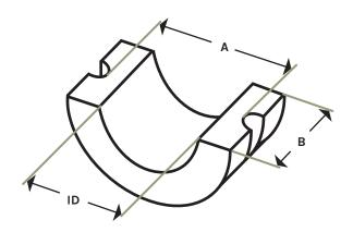
Used to support the rotating shaft in screw-conveying machinery. Ensures alignment, distributes weight, and provides smooth, low-friction rotation, even in applications involving abrasive or corrosive materials.
