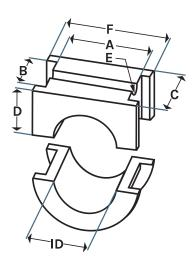
Used to support the rotating shaft in screw-conveying machinery. Ensures alignment, distributes weight, and provides smooth, low-friction rotation, even in applications involving abrasive or corrosive materials.
