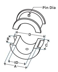
Used to support the rotating shaft in screw-conveying machinery. Ensures alignment, distributes weight, and provides smooth, low-friction rotation, even in applications involving abrasive or corrosive materials.
